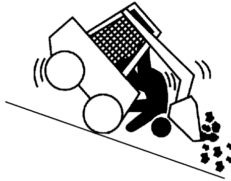
Operating On Slopes-Wheeled
